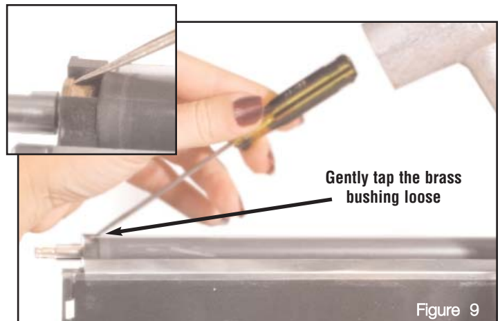
Tap the brass bushing from the slot and remove from the cartridge.
